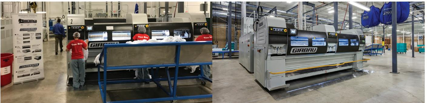
*Girbau Industrial thru-station feeders automatically straighten and feed items through a corresponding ironer.*
