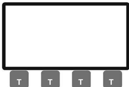
**Multi-function keyboard.** Made up of four keys (T) that execute different orders depending on what is currently in use. The function of each key is displayed on the graphic screen.
