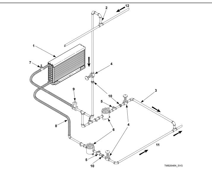
NOTE: Refer to *Table 36* for sizing of steam lines. Piping must also be sized accordingly for length of runs and number of elbows.
