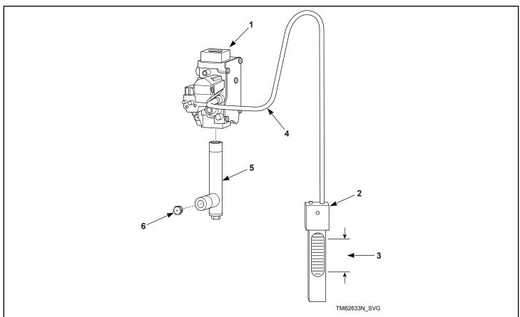
NOTE: For IEC gas valves, attach manometer to end of orifice holder. For AGA and CSA gas valves, attach manometer to the outlet pressure port on the gas valve.
