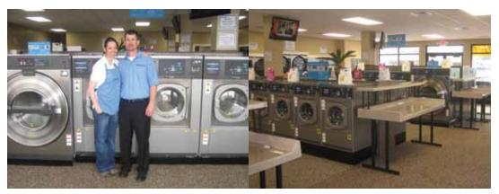
to Millman. A typical top-load washer consumes 30-40 gallons of water per load, he says. By comparison, the Express Laundry Center's 20-pound capacity ExpressWash™ Washers are front-load machines using just 13.4 gallons of water per load with quality wash results.
