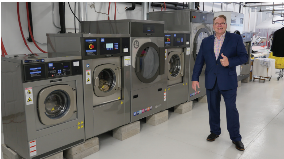
In a single shift, Paul White’s Poseidon equipment has the potential to serve 30 families and process 1,600 pounds of wetcleaned wash/dry/fold laundry per day.
