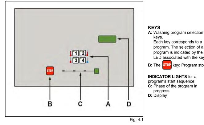
Each key corresponds to a program. The selection of a program is indicated by the LED associated with the key. B: The STOP key: Program stop. **INDICATOR LIGHTS** for a program's start sequence: C: Phase of the program in
