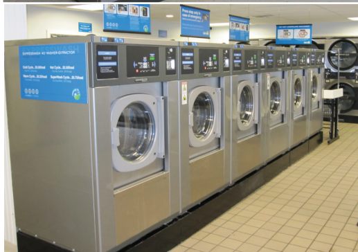
EZ Coin Op, in San Jose, Calif., (top) and Sunshine Express Laundry Center, in Salem, Mass. (bottom) recently changed out their old hard-mount machines for ExpressWash freestanding, high-speed washers.
