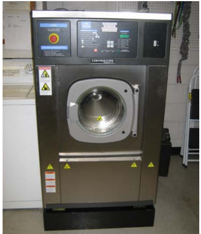
This 40-pound capacity soft-mount washer slid easily into the cramped space at Tisbury, Mass. Fire Department
