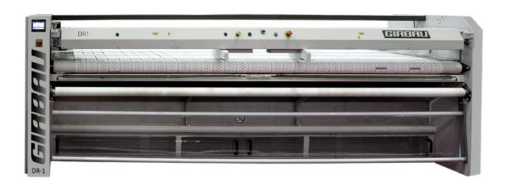
A very straightforward automatic feeder for feeding in articles automatically on 1 lane. It also allows manual feeding of items of all sizes on 1, 2 or 4 lanes.
