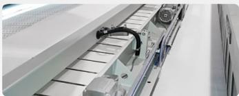
A highly recommended option for improving feeding quality even further. A number of smoothing belts located above the discharge conveyor, along with a series of brushes on 1 or 2 lanes, depending on the feeder chosen, correct any imperfections which may have appeared.
