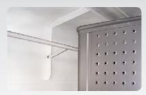
The steel rail prevents the laundry transporting carts from hitting the feeder and helps the operators to access the carts and their loads.
