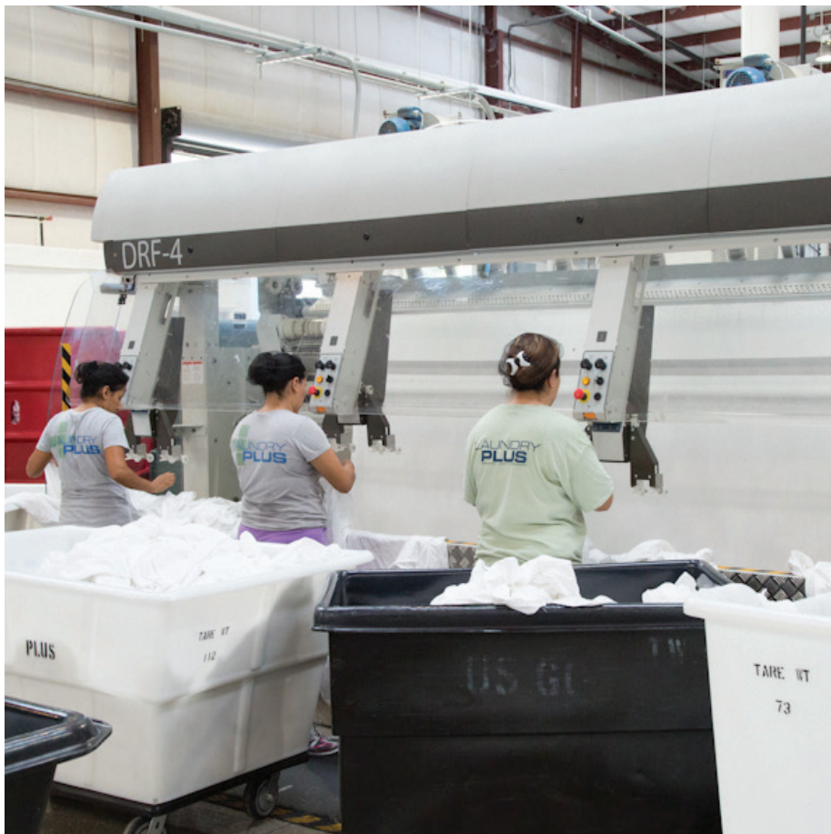
Operators clip sheets onto DRF feeder.
