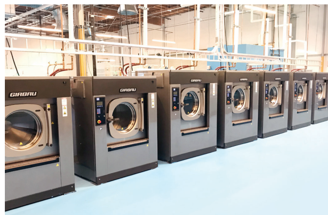
Revolve is equipped with an extensive lineup of Girbau Industrial soft-mount washers that produce extract speeds up to 387 G-force.
