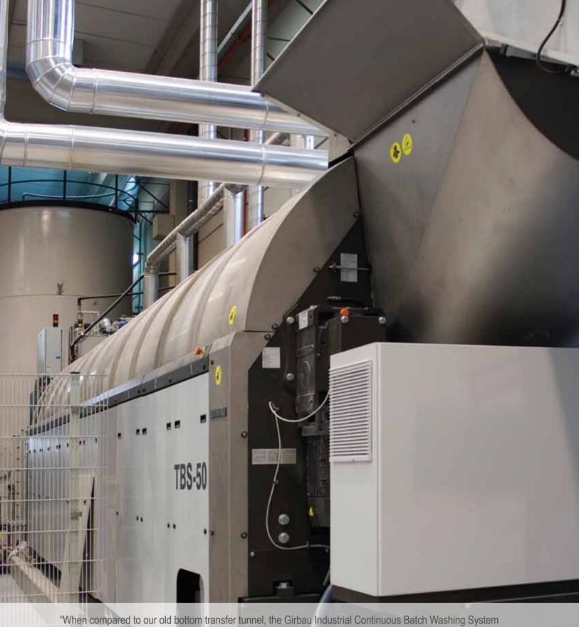
"When compared to our old bottom transfer tunnel, the Girbau Industrial Continuous Batch Washing System increased our laundry production to 3,000 pounds of laundry per hour; reduced our chemical consumption by 40 percent; and decreased our water consumption from 1.2 to .7 gallons per laundry pound versus our bottom transfer tunnel. The Girbau Industrial tunnel has been fantastic. In 13 years and thousands of operating hours, I've only done two upgrades."
