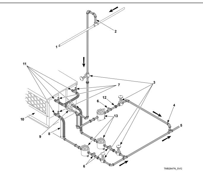
NOTE: Refer to *Table 21* for sizing of steam lines. Piping must also be sized accordingly for length of runs and number of elbows.
