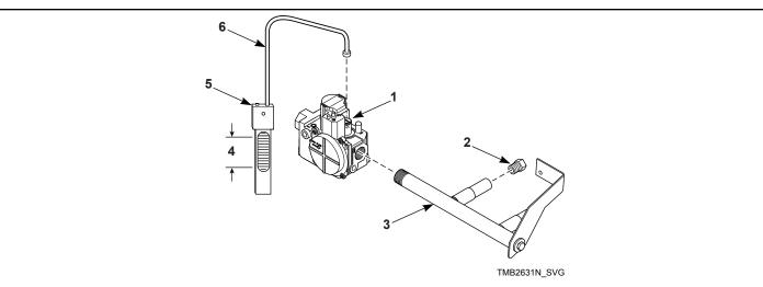
NOTE: For IEC gas valves, attach manometer to end of orifice holder. For AGA and CSA gas valves, attach manometer to the outlet pressure port on the gas valve.
