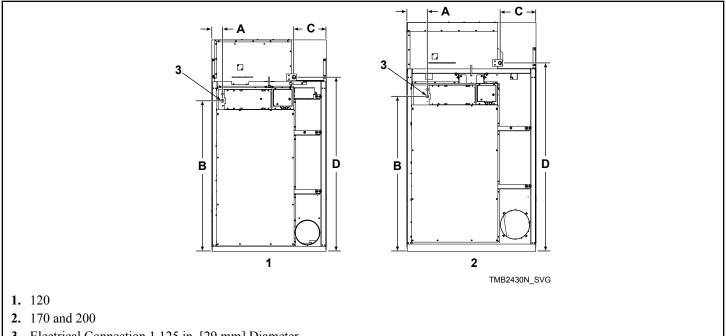
**3.** Electrical Connection 1.125 in. [29 mm] Diameter
