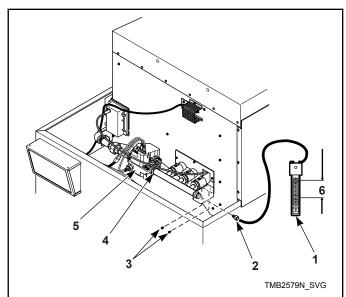
NOTE: For IEC gas valves, attach manometer to end of orifice holder. For AGA and CSA gas valves, attach manometer to the outlet pressure port on the gas valve.
