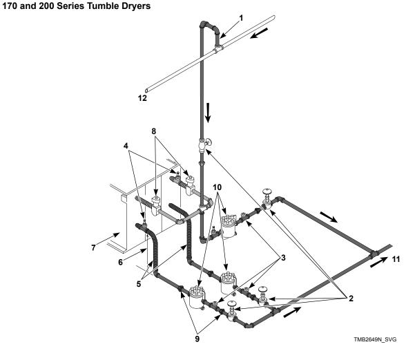
NOTE: Refer to *Table 12* for sizing of steam lines. Piping must also be sized accordingly for length of runs and number of elbows.
