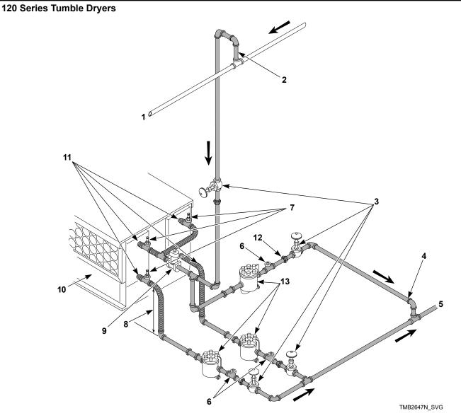
NOTE: Refer to  $Table\ 11$  for sizing of steam lines. Piping must also be sized accordingly for length of runs and number of elbows.
