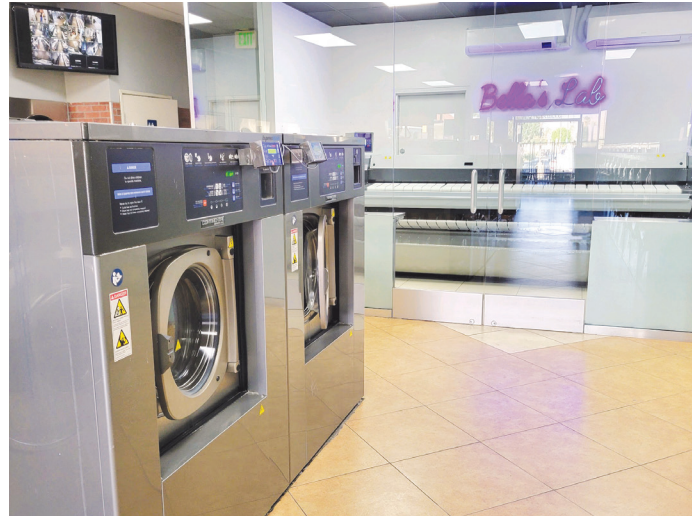
Left: Sparklean made smart equipment tweaks to better serve the booming vacation rental market. Right: The laundry installed a heated-roll Continental Express Ironer and two 80-pound capacity Continental ExpressWash® washers with automatic chemical injection.
