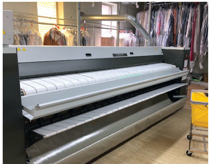
The Poseidon Ironer is situated in a small, 200-square-foot area, it processes linens straight from the washer while they're still damp.
